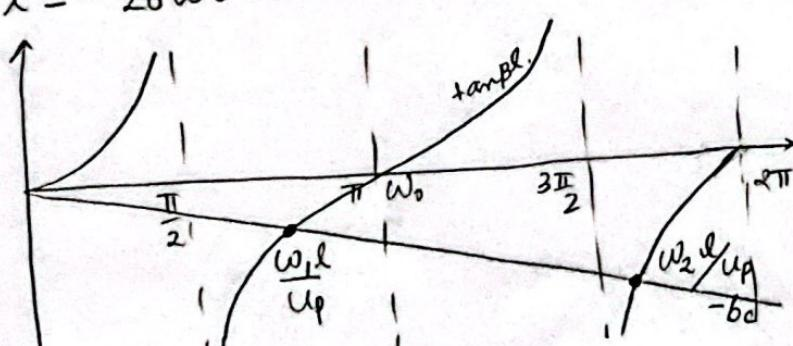
Gap coupling reduces the resonant frequency from  $\omega_0 \rightarrow \omega_1$ . If  $b_c \ll l \Rightarrow \omega_1$  is close to  $\omega_0$ .
