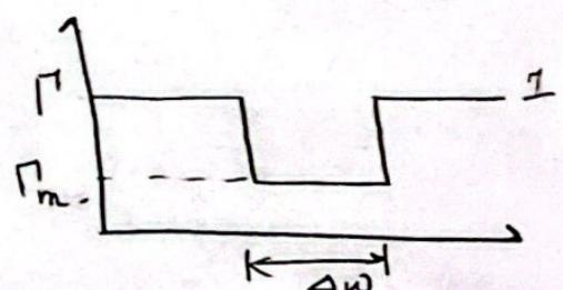
$\Gamma(\omega) = 0$  at some point  $\Rightarrow$  the width of the match must be 0.
