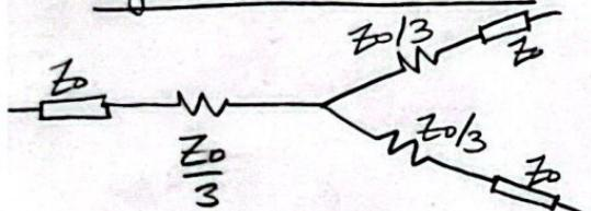
$$S = \begin{bmatrix} 0 & \frac{1}{2} & \frac{1}{2} \\ \frac{1}{2} & 0 & \frac{1}{2} \\ \frac{1}{2} & \frac{1}{2} & 0 \end{bmatrix} \rightarrow \begin{aligned} &6\text{dB insertion loss.} \\ &\frac{1}{4} \text{ power split by } \omega \text{ & } 2 \\ &\frac{1}{2} \text{ power dissipated.} \\ &\Rightarrow \text{High bandwidth.} \\ &\Rightarrow \text{Measurement devices.} \end{aligned}$$
