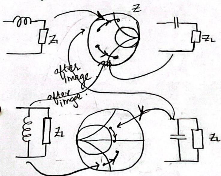
Move along constant VSWR circle in clockwise direction when extending the line length (electrical length).
