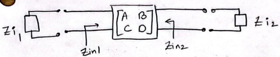
→ If connecting  $Z_{i1}$  &  $Z_{i2}$  ensures  $Z_{in1} = Z_{i1}$  &  $Z_{in2} = Z_{i2}$
