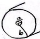
$$\phi(p, \phi) = \frac{V_0 \ln b/p}{\ln b/a} \quad \text{for TEM mode.}$$
