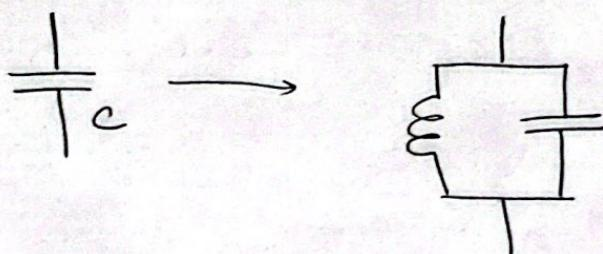
$$L_k' = \frac{\Delta Z_0}{\omega_0 C_k \rightarrow g_k} \\ C_k' = \frac{C_k \rightarrow g_k}{\Delta \omega_0 Z_0}$$
