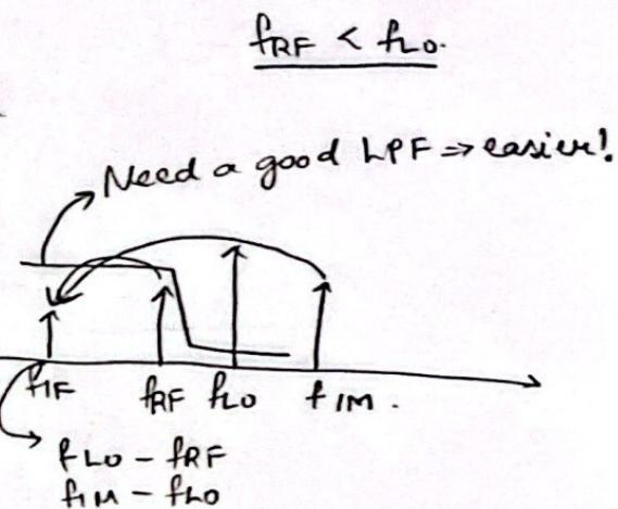
Since  $f_{LO}$  is higher than earlier,  $f_{IM}$  must be much higher to fall on fRF therefore a shallow roll off LPF does the job.
