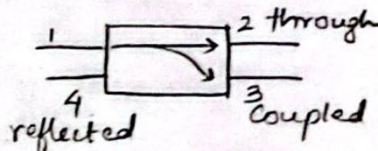
↳ determines how well coupled & reflected waves are isolated.
