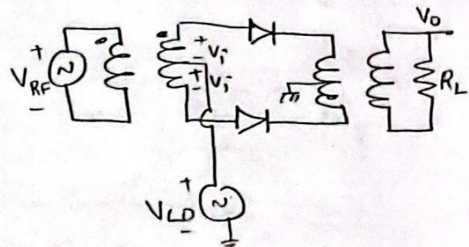
$V_{LO} > 0 \Rightarrow$  Both diodes are ON  $\Rightarrow V_o = V_i$
