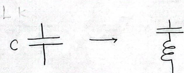
$$L_k' = \frac{Z_0}{\omega_0 \Delta C_k} \\ C_k' = \frac{\Delta C_k}{\omega_0 Z_0}$$
