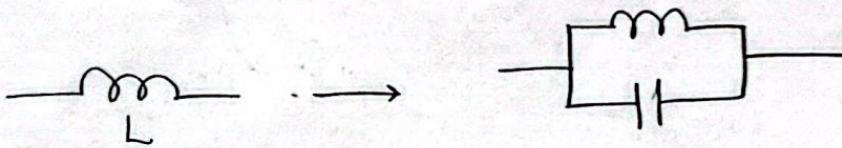
$$L_k' = \frac{\Delta L_k Z_0}{\omega_0} \\ C_k' = \frac{1}{\omega_0 \Delta L_k Z_0}$$
