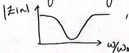
b) Input impedance of parallel resonator
