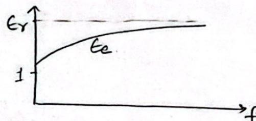
Filling Factor (portion of EM energy inside the substrate)
