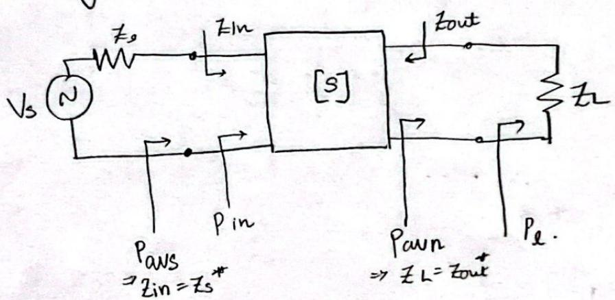
$$P_{\text{in}} = \frac{|V_s|^2}{8Z_0} \frac{|1 - \Gamma_S|^2}{|1 - \Gamma_{\text{in}} \Gamma_S|^2} (1 - |\Gamma_{\text{in}}|^2)$$
