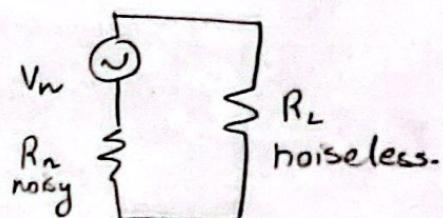
Equivalent noise temperature → (sensitive scale used in astronomy)
