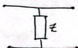
$[S] = \begin{bmatrix} -\frac{Z_0}{2Z+Z_0} & \frac{2Z}{2Z+Z_0} \\ \frac{2Z}{2Z+Z_0} & \frac{-Z_0}{2Z+Z_0} \end{bmatrix}$
