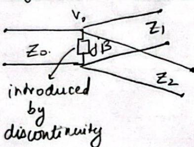
$$P_{in} = \frac{1}{2} \frac{V_0^2}{Z_0^2} \quad P_1 = \frac{1}{2} \frac{V_0^2}{Z_1} \quad P_2 = \frac{1}{2} \frac{V_0^2}{Z_2}$$
