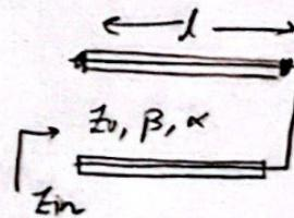
$$\Rightarrow R = \frac{Z_0}{\alpha l}, \quad C = \frac{1}{j \omega_0 Z_0}, \quad \Theta = \omega_0 R C \Rightarrow \boxed{\Theta = \frac{\beta}{2 \alpha}}$$
