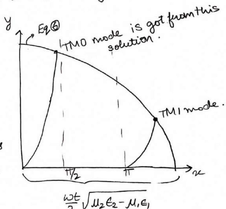
→ There is no cut off for TM<sub>0</sub> mode propagation.
