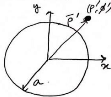
The scattered wave must satisfy the B.C:  $\psi_i(a, \phi) + \psi_s(a, \phi) = 0$
