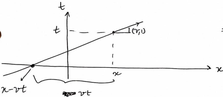
$$\begin{aligned} \Rightarrow u(x, t) &= u(x - vt, 0) \\ &= u_0(x - vt) \end{aligned}$$
